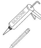
Cut out worktop to supplied dimensions shown (fig. 1) with suitable equipment. Seal the cut edge of the worktop using silicone or PTFE and allow to dry prior to fitting the hob.
