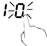
3. Using the "+" or "-" buttons ,you can realize the setting of timing from 1 to 99 minutes.
